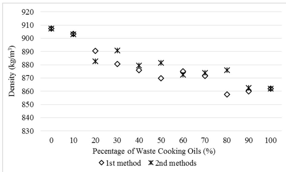
**Figure 1.** Density of biodiesel mixture of *Jatropha* seed oil and waste cooking oil.
