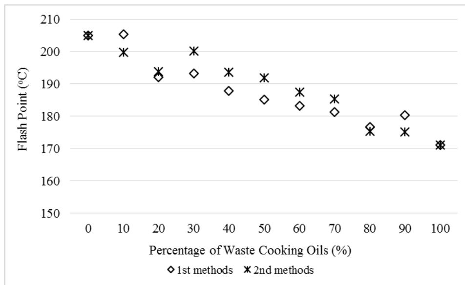
Figure 3. Flash point of biodiesel mixture.
