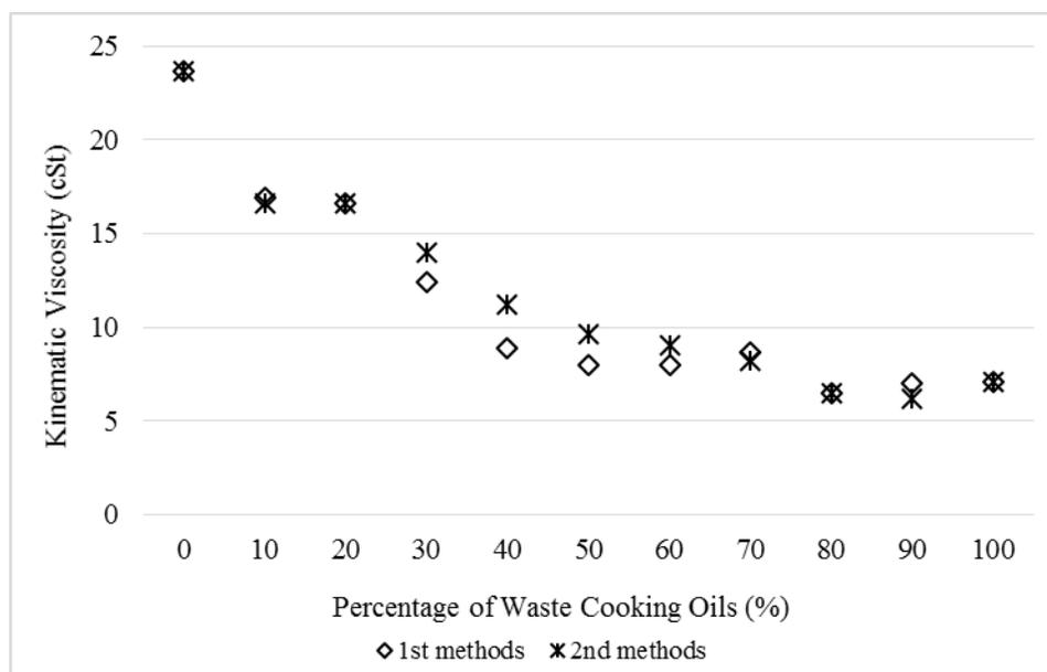
**Figure 2.** Viscosity of biodiesel mixture of *Jatropha* seed oil and waste cooking oil.
