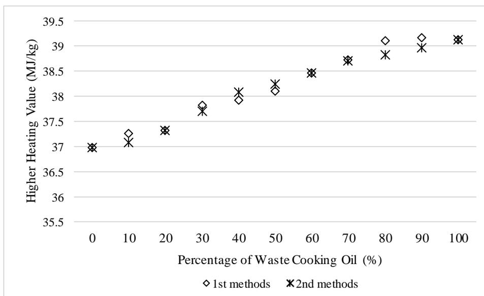
Figure 4. Calorific value of biodiesel mixture.
