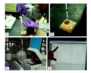
Figure 1. A-D showing the steps of working with a Lab on a Chip and analyzing data. A. Loading the sample to the Chip. B. A chip loaded with sample. C. The Chip placed into the Bioanalyzer. D. Computer screen showing the Electropherogram.
