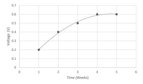
Figure 1. Development of the open circuit voltage of the MFC over a month.
