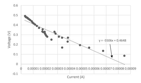
Figure 5. Current-Voltage plot for the MFC used for calculating the internal resistance.
