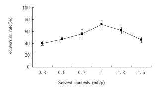
**Figure 12.** Effect of organic solvent contents on biodiesel conversion.
