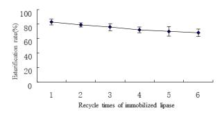
**Figure 9.** Effect of recycle times of immobilized lipase on esterification rate of artificial sour oil.
