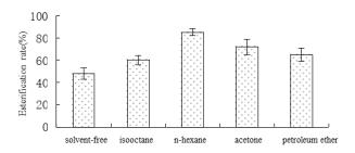
$\label{lem:figure 3.} \textbf{Effect} of different solvent on esterification rate of artificial sour oil.$
