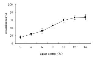
Figure 10. Effect of lipase contents on biodiesel conversion.
