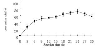
Figure 13. Effect of reaction time on biodiesel conversion.
