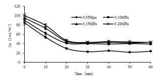
Figure 2. Effect of operating pressure on membrane flux.
