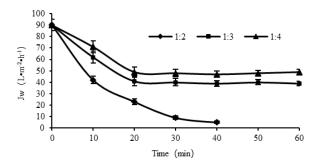
Figure 1. Effect of dilution on membrane flux.
