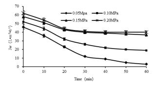
Figure 9. Effect of operating pressure on membrane flux.
