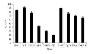
Figure 3. Adsorption capacity of different resins to lysozyme.
