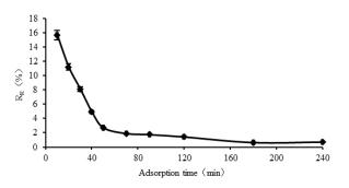
Figure 6. Effect of adsorption time on lysozyme adsorption.
