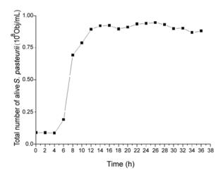
Figure 1. Growth curve of S. pasteurii.
