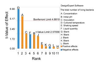
Figure 3. Pareto chart of each factor standard effect on the number of living *S. pasteurii*.
