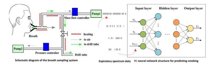
Figure 1. Framework for predicting the smoking behavior by combining exhalation mass spectrometry with a fully connected neural network.
