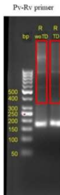
Figure 2. PCR products of both standard (R wo TD) and touchdown PCR (R TD) assays using Pv-Rv primers. The red box indicated the background intensity.
